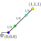
Use our observations about resistors in series to collapse these three edges into one edge:
