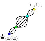
Use our observations about resistors in parallel to collapse these multiple edges to single edges:
