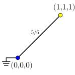
Now, apply Ohm's law to deduce that  $i_{\text{source}} = (v(\text{source}) - v(\text{sink})/R_{\text{eff}} = 6/5$ , and therefore that  $p_{\text{esc}} = \frac{6/5}{C_{\text{source}}} = \frac{6/5}{3} = 2/5$ . (Recall that  $C_{\text{source}}$  is just the sum of the conductances of the edges leaving the source. In particular, because there are three edges leaving the origin all with resistance 1, this is just  $\frac{1}{1} + \frac{1}{1} + \frac{1}{1} = 3$ .) So our probability of escape is 2/5!
