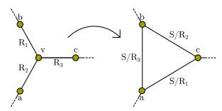
The star-triangle transformation. In the above diagram,  $S = R_1 R_2 + R_1 R_3 + R_2 R_3$ .
