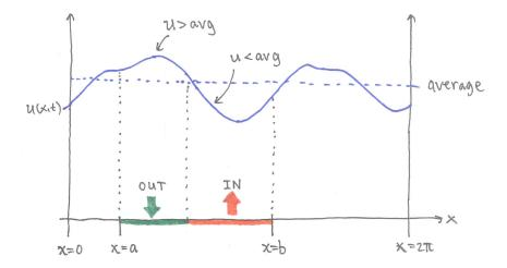
Figure : Notional depiction of distributed pumping over interval.
